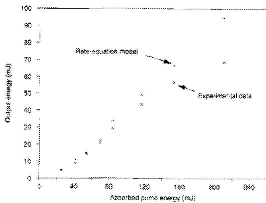
Fig. 6. Comparison of calculated and experimental input/output data for a Co:MgF<sub>2</sub> laser operating at room temperature.
