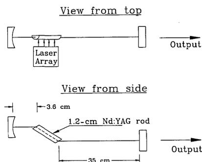
Fig. 2. Schematic layout of the laser resonator.
