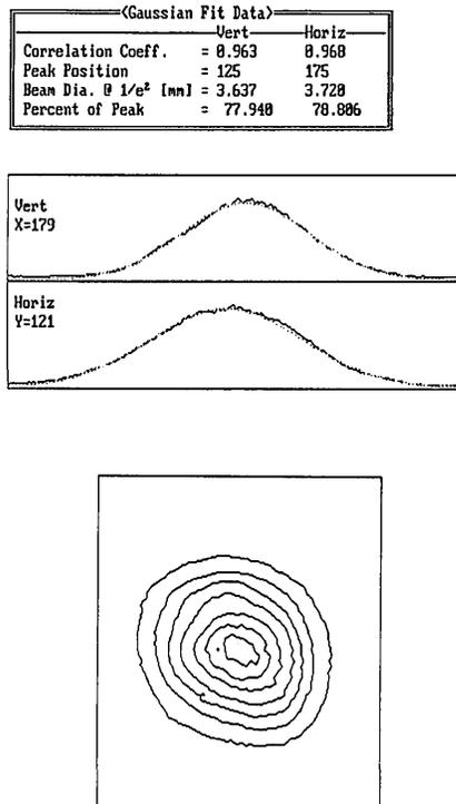
Fig. 4. Contour plot and beam profiles for the TEM<sub>00</sub>-mode output beam.
