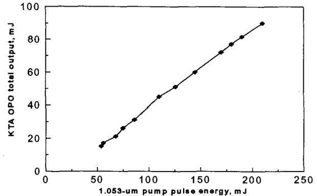
Figure 3. Input/output data for KTA OPO.
