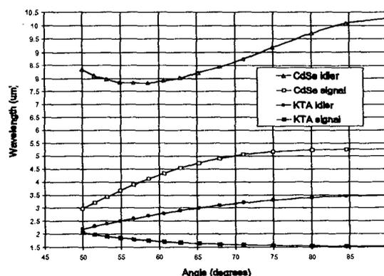
Figure 1. Composite angle-tuning for KTA-CdSe tandem OPO.
